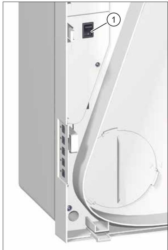
Fig. 18: Mains switch, visible when unit cover is removed
