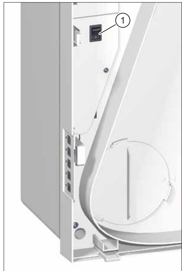
Fig. 14: Mains switch, visible when unit cover is removed
